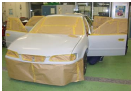
塗装作業(全塗装)
